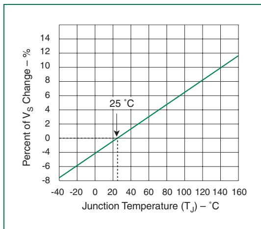
**Normalized V<sub>S</sub> Change versus Junction Temperature**
