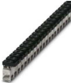
Power terminal block, Connection method Screw connection, Load current : 125 A, Cross section: 2.5 mm 2 - 35 mm 2 , Width: 14.3 mm, Color: black
