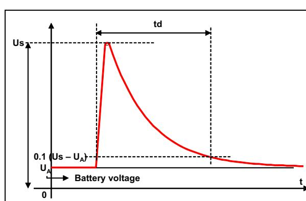
**Figure 10. Load dump capability (LDP01-30AY
