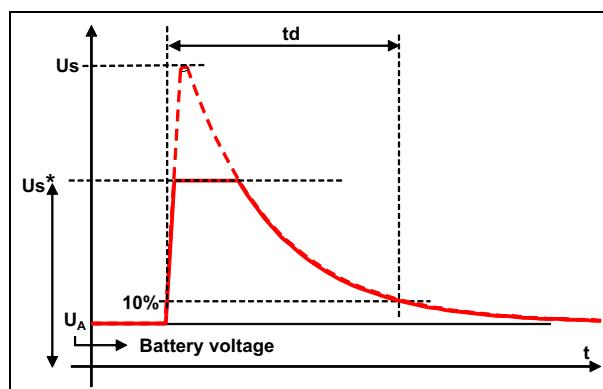
**Figure 12. Load dump capability (LDP01-30AY)**
