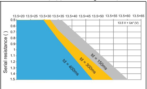
**Figure 9. ISO 16750-2, test A definition**
