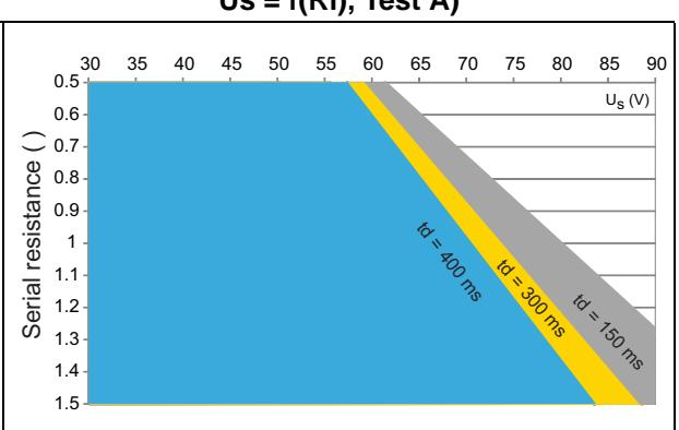
**Figure 11. ISO 16750-2, test B definition**
