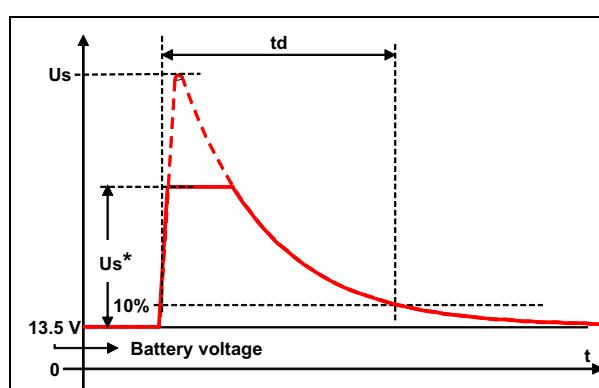
**Figure 8. Load dump capability (LDP01-30AY
