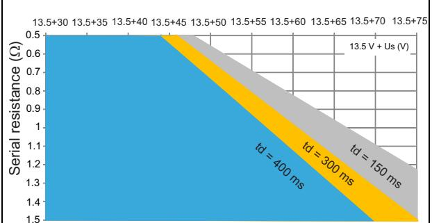
**Figure 7. ISO7637-2, pulse 5b definition**
