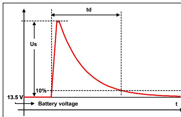
**Figure 6. Load dump capability (LDP01-30AY
