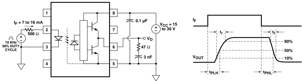
Figure 17. Propagation delay test circuit and waveforms.
