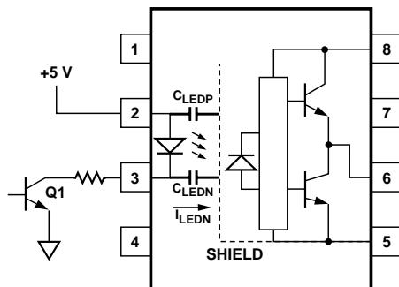
Figure 24. Not recommended open collector drive circuit.
