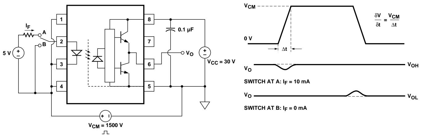
Figure 18. CMR test circuit and waveforms.
