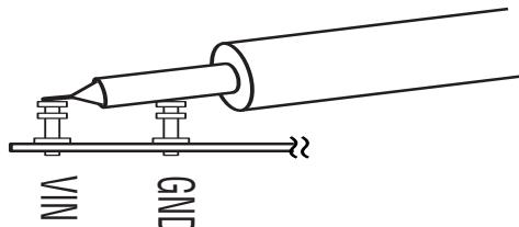
**Figure 3. Measuring Input or Output Ripple**
