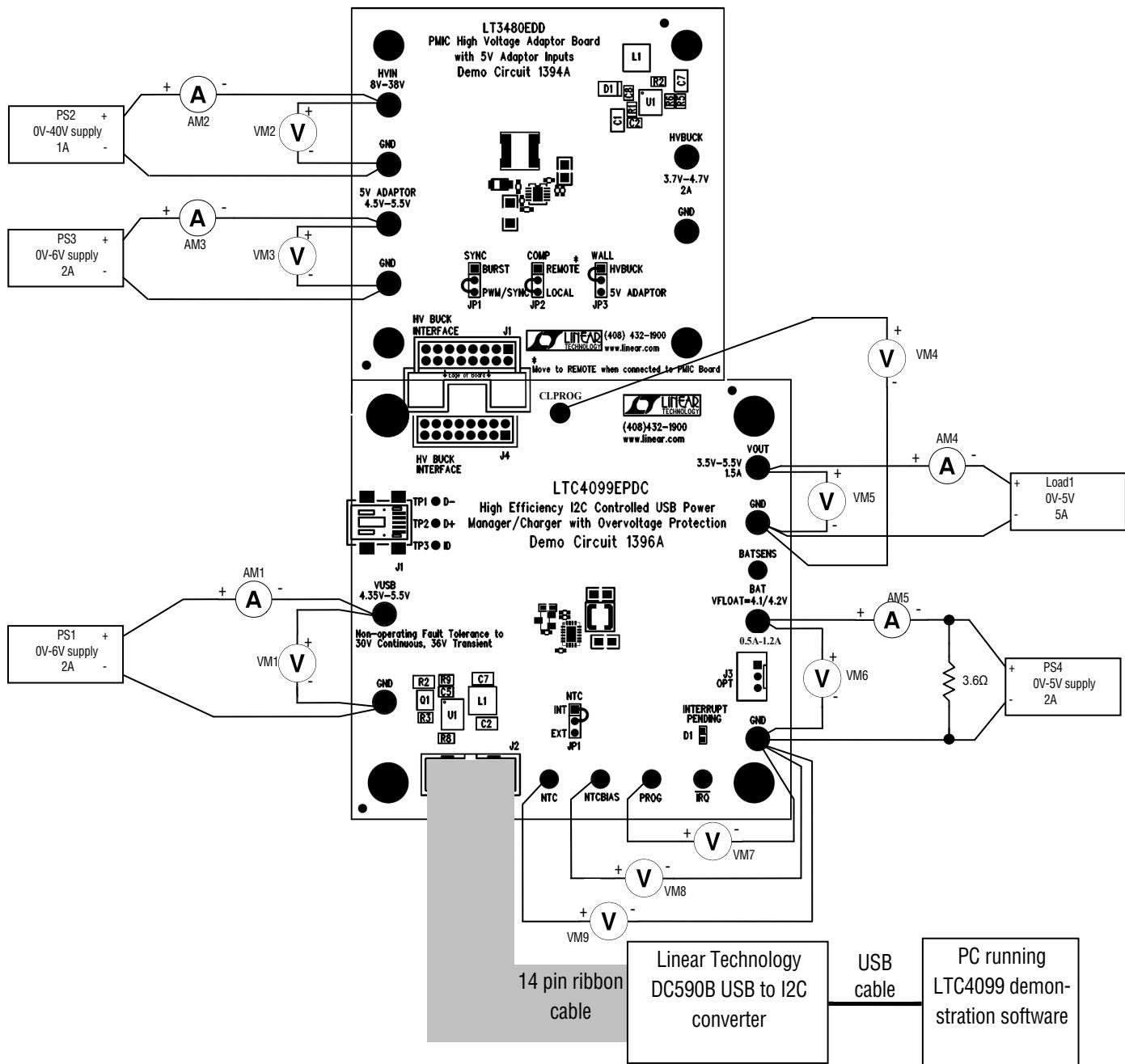
Note: All connections from equipment should be Kelvin connected directly to the Board PINS which they are connected to on this diagram and any input, or output, leads should be twisted pair
