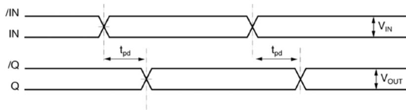
Figure 1a. Propagation Delay
