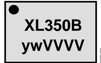
Figure 2. Product Information on Package (Top View)
