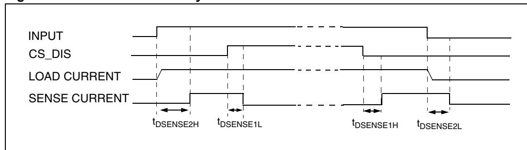
**Figure 5. Switching characteristics**
