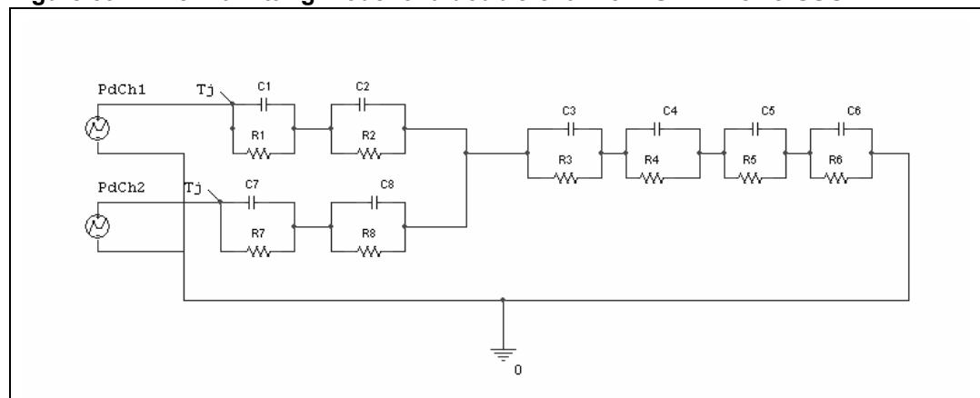
1. The fitting model is a simplified thermal tool and is valid for transient evolutions where the embedded protections (power limitation or thermal cycling during thermal shutdown) are not triggered.
