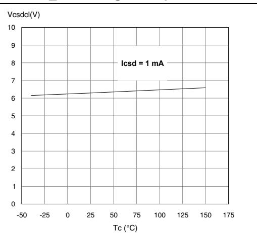
**Figure 28.** Low-level CS\_DIS voltage
