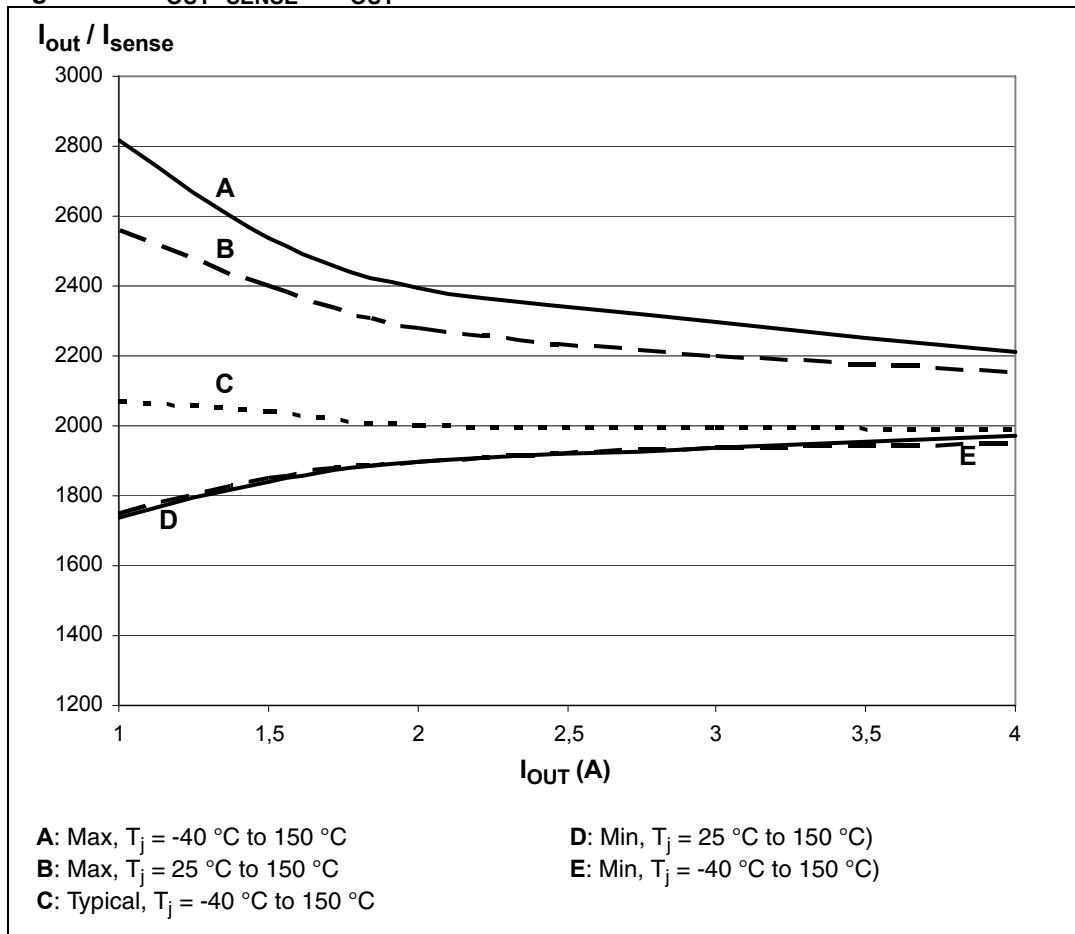
**Figure 9.** Maximum current sense ratio drift vs load current<sup>(1)</sup>
