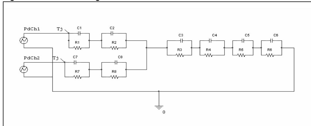
1. The fitting model is a simplified thermal tool and is valid for transient evolutions where the embedded protections (power limitation or thermal shutdown during thermal shutdown) are not triggered.
