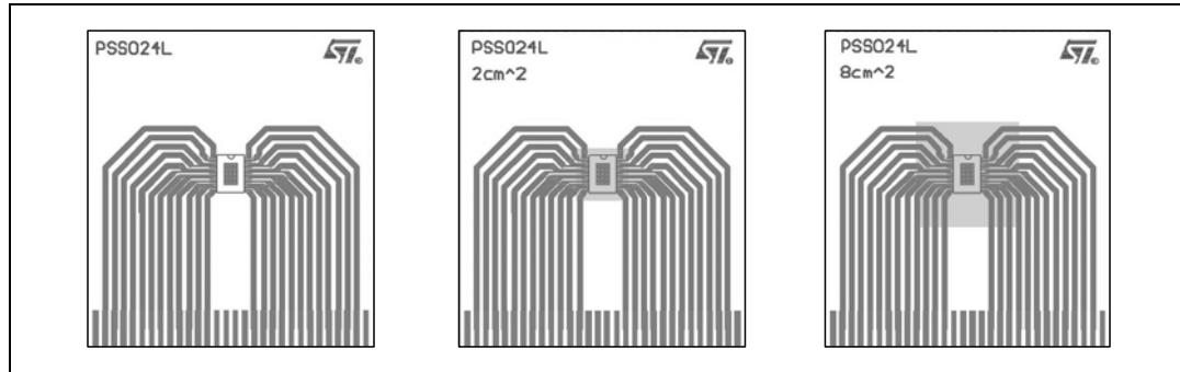
1. Layout condition of  $R_{th}$  and  $Z_{th}$  measurements (PCB: double layer, Thermal vias, FR4 area = 77 mm x 86 mm, PCB thickness = 1.6 mm, Cu thickness = 70  $\mu$ m (front and back side), Copper areas: from minimum pad lay-out to 8  $\text{cm}^2$ ).
