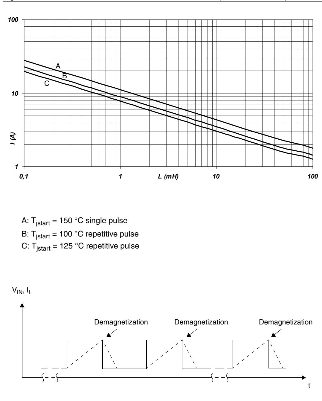
1. Values are generated with  $R_L = 0 \Omega$ . In case of repetitive pulses,  $T_{jstart}$  (at beginning of each demagnetization) of every pulse must not exceed the temperature specified above for curves A and B.
