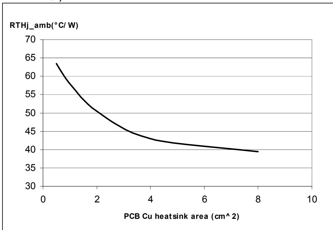
**Figure 34.** PowerSSO-12 thermal impedance junction ambient single pulse (one channel on)
