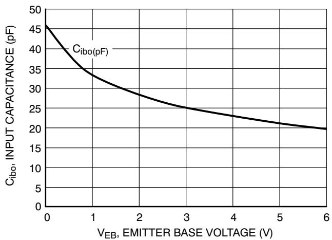
**Figure 8. Input Capacitance**
