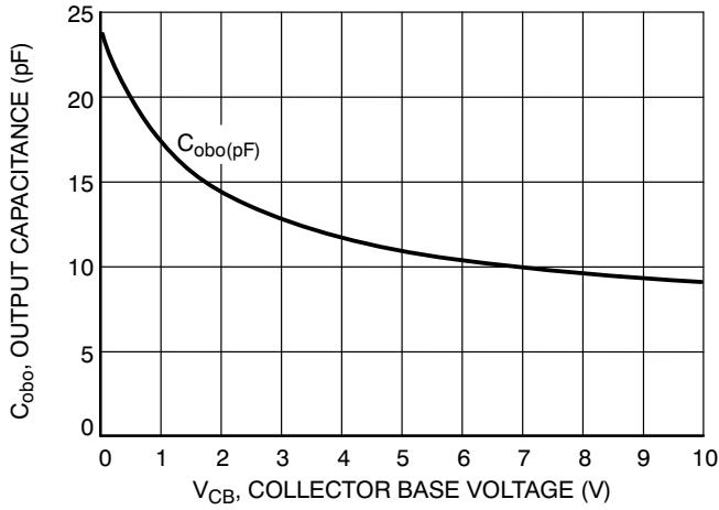
**Figure 9. Output Capacitance**
