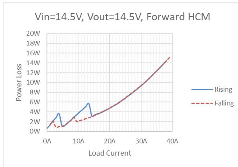
Figure 2. Power Loss in Forward HCM Buck-Boost Mode as Function of Load Current.  $V_{IN} = V_{OUT} = 14.5V$ . Constant Current Load Connected to  $V_{OUT}$ . The Measurement is Done by Increasing Load Current (Blue Line) Until Current Limit, then Decreasing the Current to Zero (Red Line)
