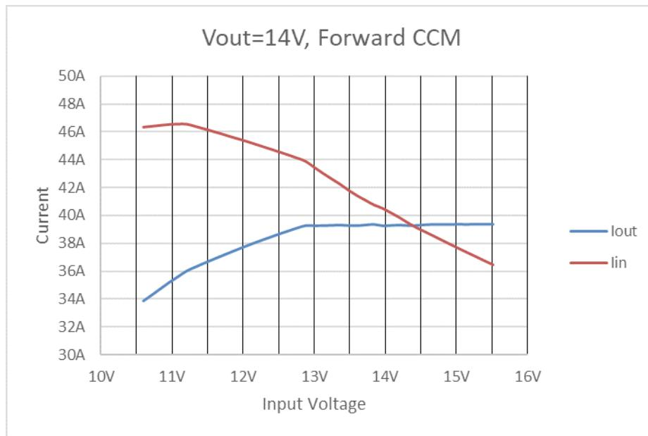
Figure 1. Input and Output Currents as Function of Input Voltage, with a Constant Voltage Load Set at 14.0V Connected to  $V_{OUT}$ . Forward CCM Mode. Output Current is Lower than Set Point when  $V_{IN}$  is Below 13V Because the Input Current Limit is Activated
