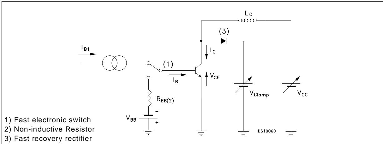
**Figure 2:** Resistive Load Switching Test Circuit.
