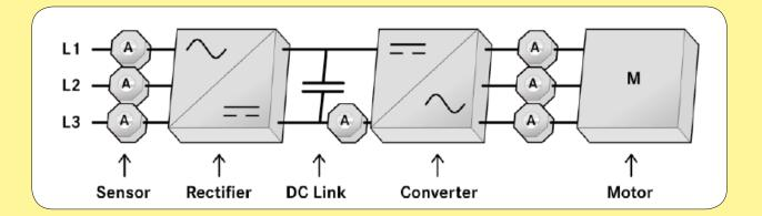
• Frequency converter for Generator-Grid connection
