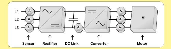
Frequency converter for Generator-Grid connection
