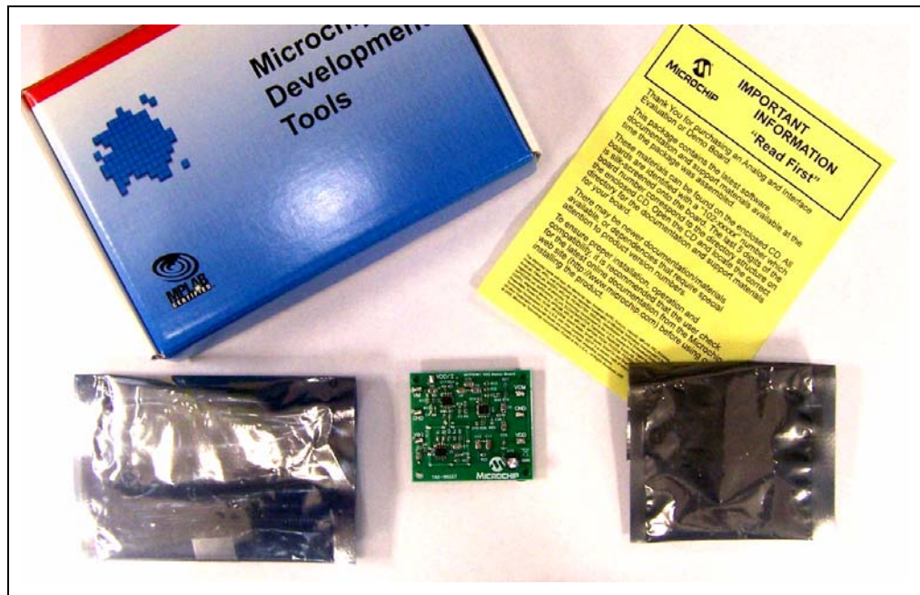
FIGURE 1-1: MCP6V01 Input Offset Demo Board Contents.
