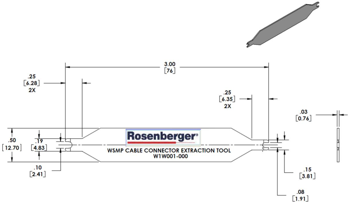
All dimensions are in inches [mm]; tolerances according to ISO 2768 m-H
