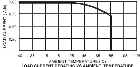
**LOAD CURRENT DERATING VS AMBIENT TEMPERATURE**
