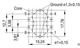
Hole arrangement View in mounting direction
