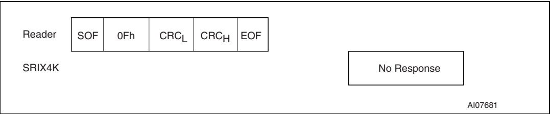
Figure 38. Completion frame exchange between reader and SRIX4K
