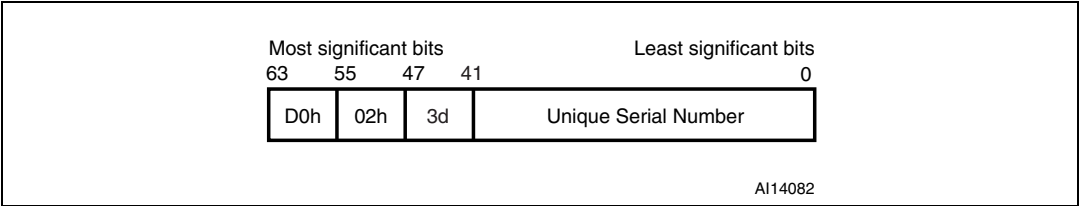
Figure 50. 64-bit unique identifier of the SRIX4K
