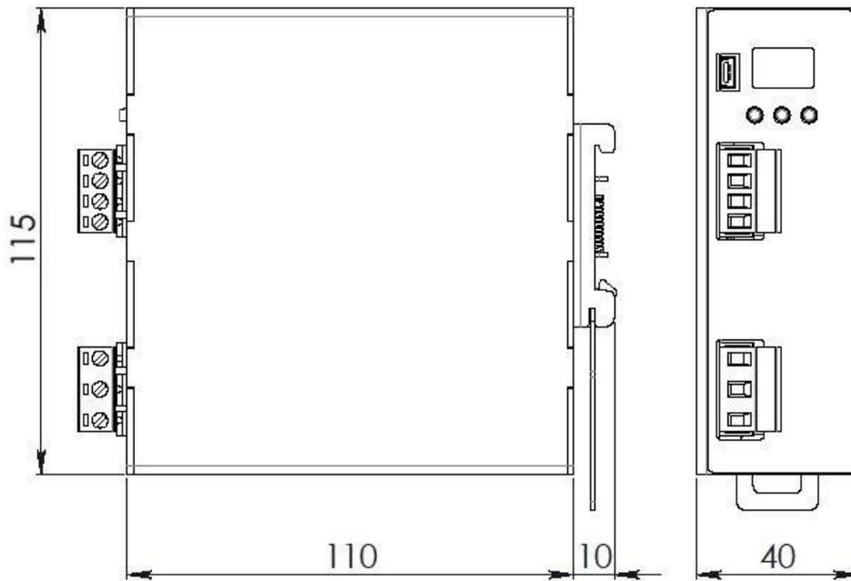
Figure 3. Mechanical Drawing
