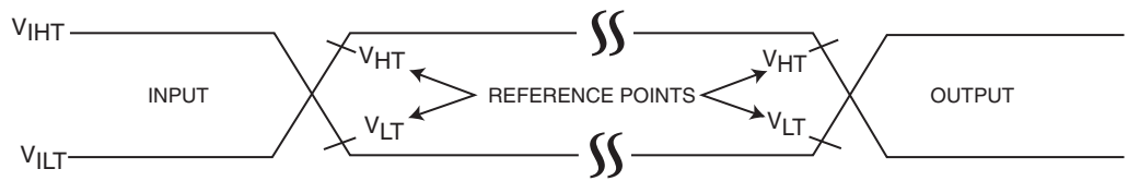
FIGURE 6-7: AC INPUT/OUTPUT REFERENCE WAVEFORMS
