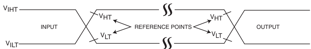
FIGURE 6-7: AC INPUT/OUTPUT REFERENCE WAVEFORMS
