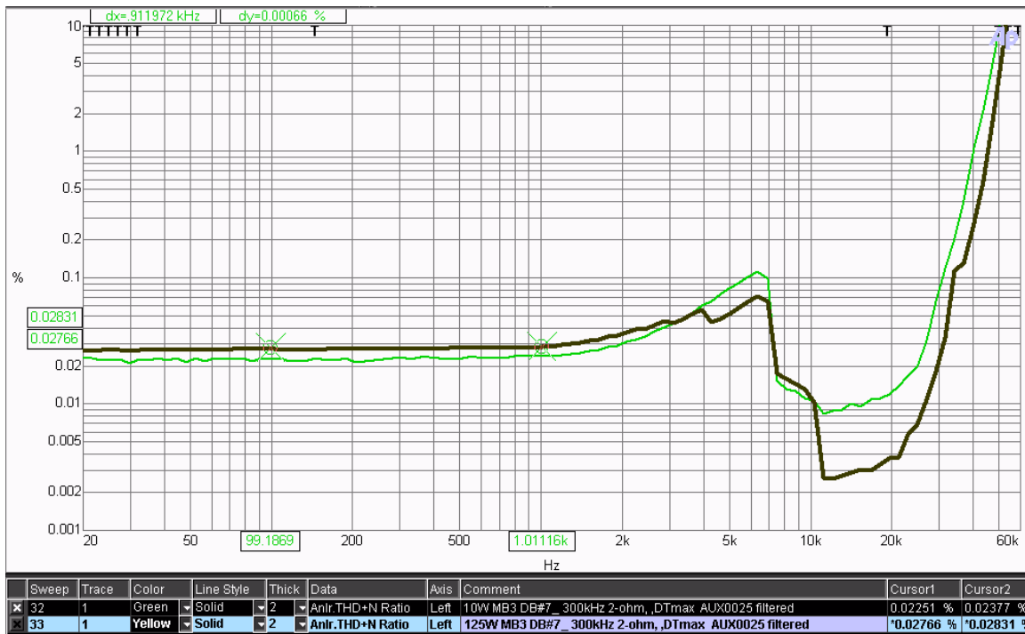
Figure 4 THD+N vs. Frequency at 10W and 125W
