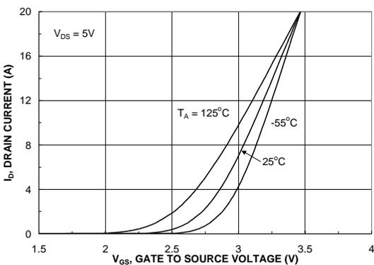
Figure 5. Transfer Characteristics.
