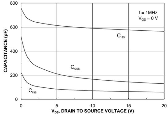
Figure 8. Capacitance Characteristics.
