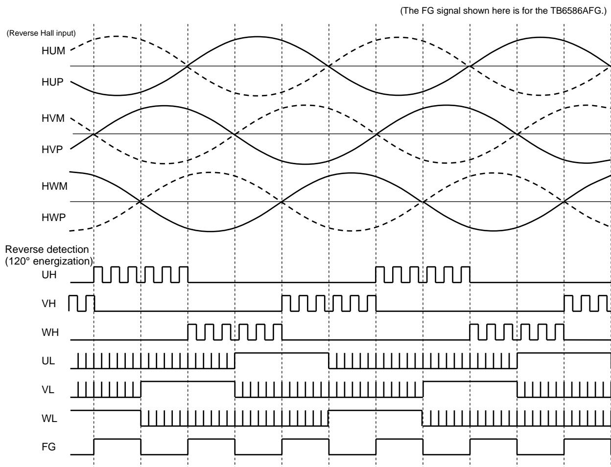
\*: When CW/CCW = Low and a reverse Hall signal is input, the motor runs at 120° energization for a lead angle of 0° ("headwind" operation)
