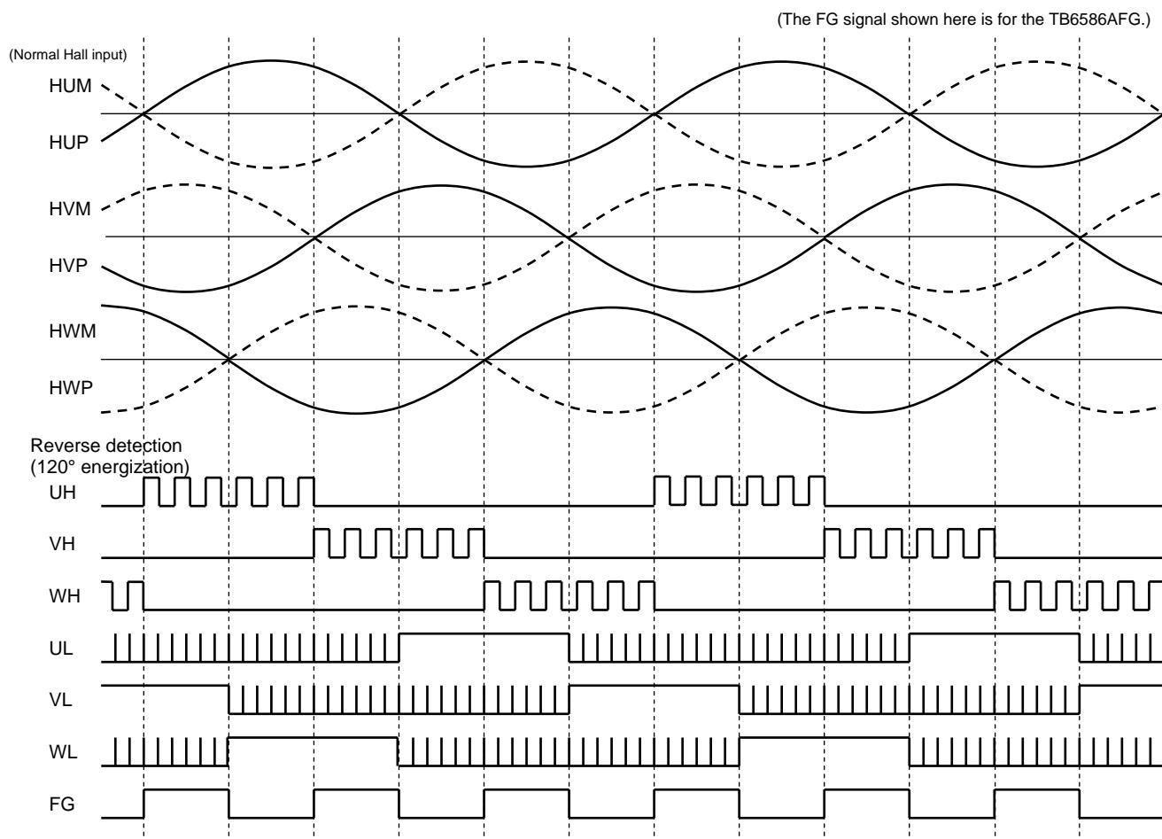
\*: When CW/CCW = Low and a reverse Hall signal is input, it runs at 120° energization for a lead angle of 0° ("headwind" operation).
