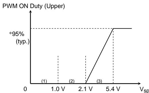
\*: The maximum ON duty is  $T_{on} = 95\%$  (typ.) when  $V_{SP} = 5.4$  V (typ.).
