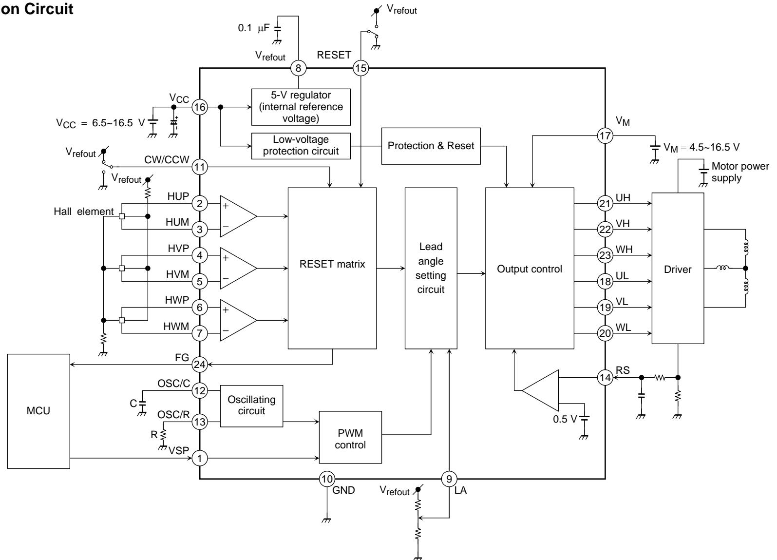
Any short circuit between the outputs, or between output and supply or ground, may damage the device. Peripheral parts may also be damaged by overvoltage and overcurrent. Design the output lines, V<sub>CC</sub>, VM and GND lines so that short circuits do not occur.
