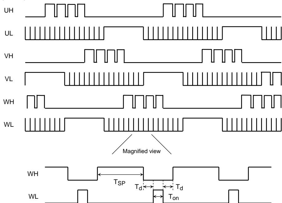
$T_{SP}$ : Variable depending on the V<sub>SP</sub> (the figure above being applicable when V<sub>SP</sub> = 5.4 V (typ.));  $T_{on} = 18/f_{osc}$ ;  $T_d = 18/f_{osc}$
