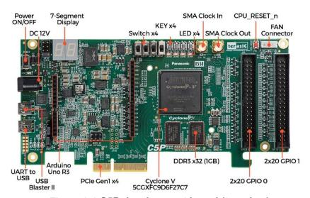
Figure 2-1 C5P development board (top view)
