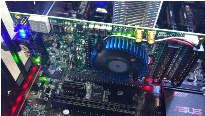
Figure 7-8 FPGA board installation on PC
