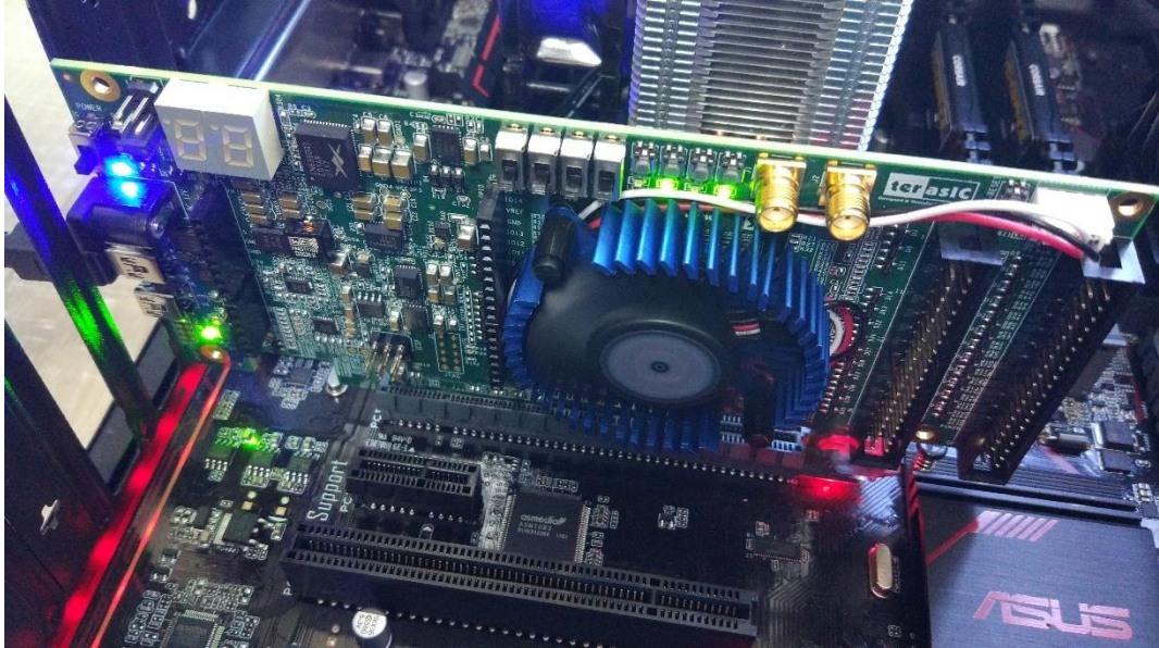
Figure 8-4 FPGA board installation on PC
