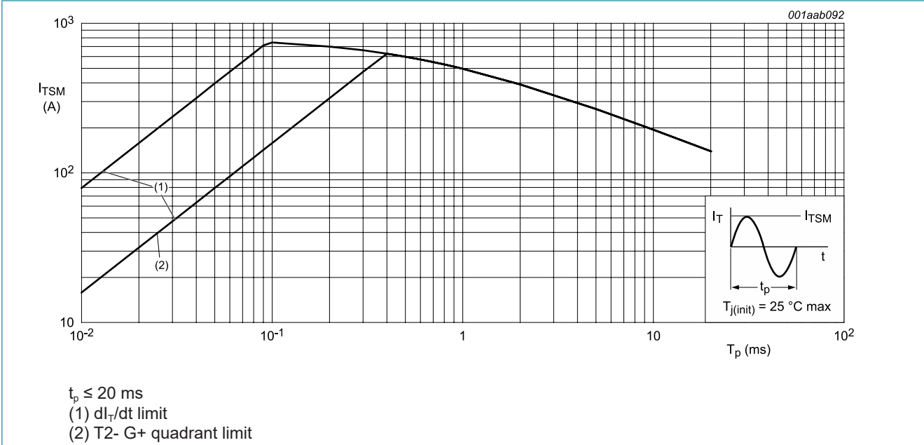
Fig. 4. Non-repetitive peak on-state current as a function of pulse width; maximum values
