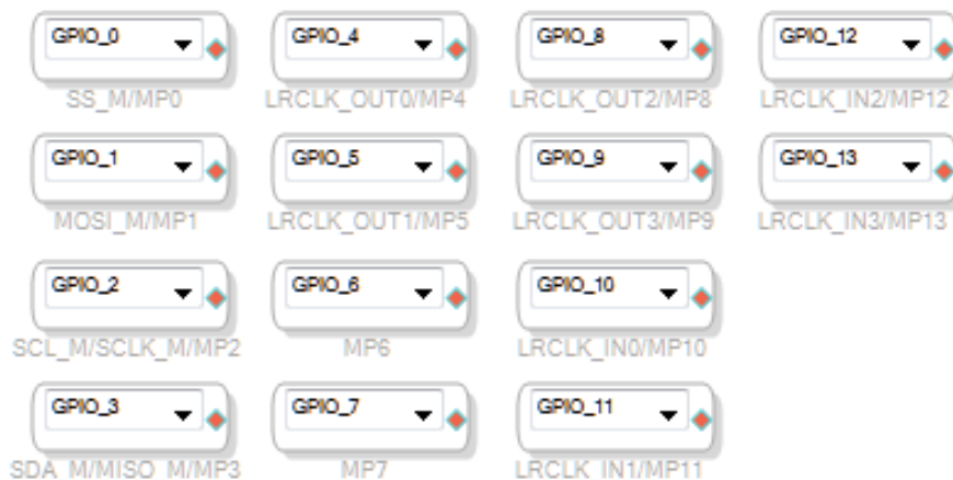
Figure 75. Complete Set of General-Purpose Inputs in SigmaStudio
