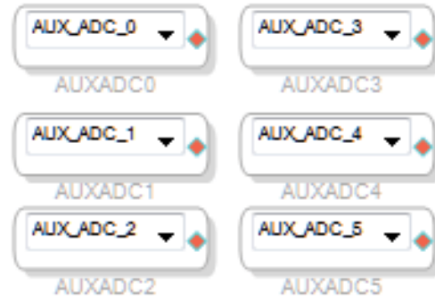
Figure 78. Complete Set of Auxiliary ADC Inputs in SigmaStudio
