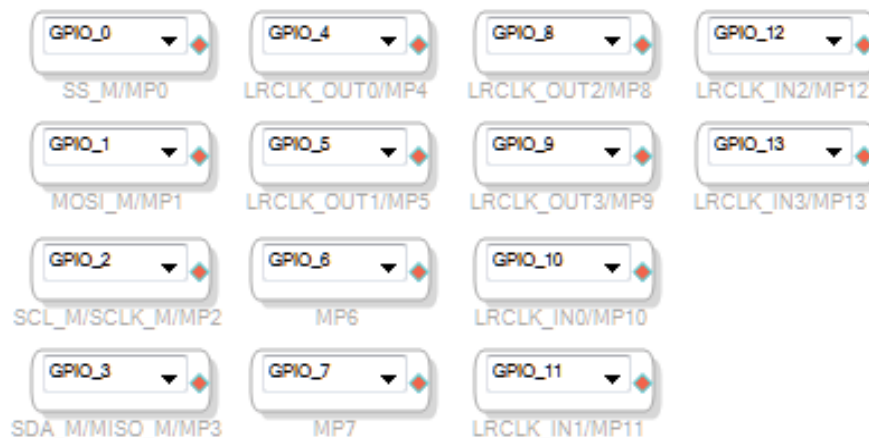
Figure 75. Complete Set of General-Purpose Inputs in SigmaStudio
