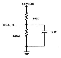
\* INCLUDING SCOPE AND JIG CAPACITANCE
