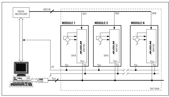
Figure 7. Automated Test System Concept
