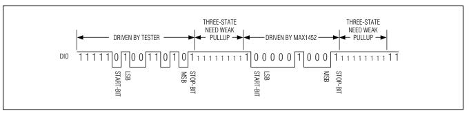
Figure 5. DIO Output Data Format
