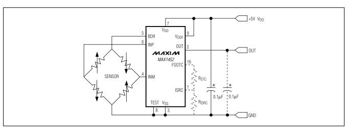
Figure 2. Basic Ratiometric Output Configuration
