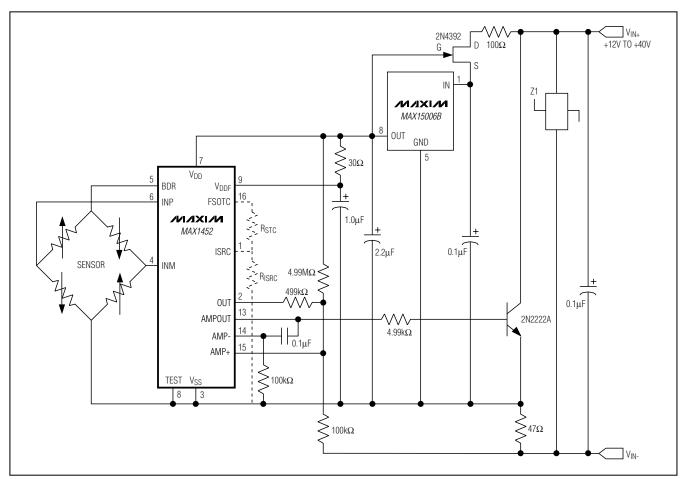
Figure 4. Basic 4–20mA Output, Loop-Powered Configuration
