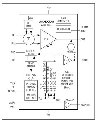
Figure 1. Functional Diagram
