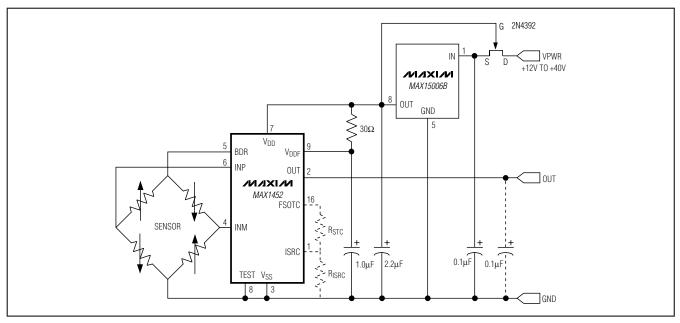
Figure 3. Basic Nonratiometric Output Configuration
