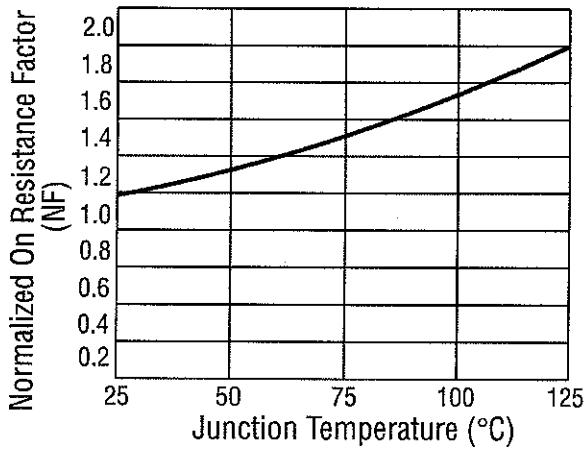
Figure 5 - Temperature Derating Curve
