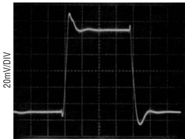
Small-Signal Transient Response V_S = \pm 2.5V
