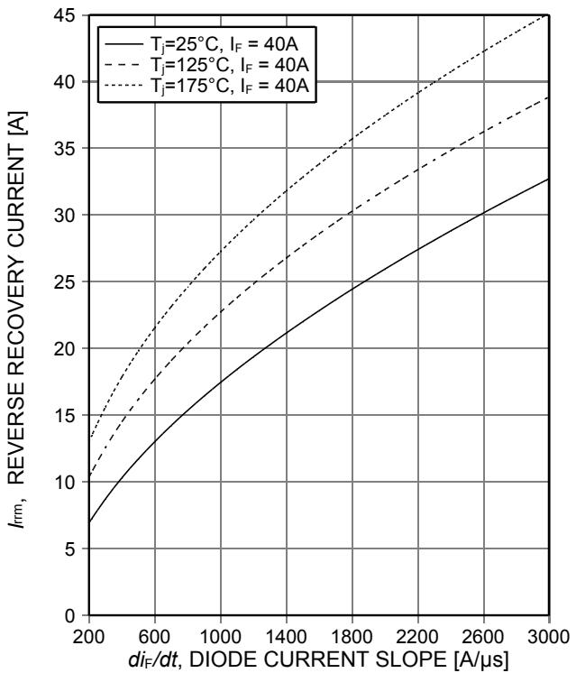
Figure 6. Typical peak reverse recovery current as a function of diode current slope
