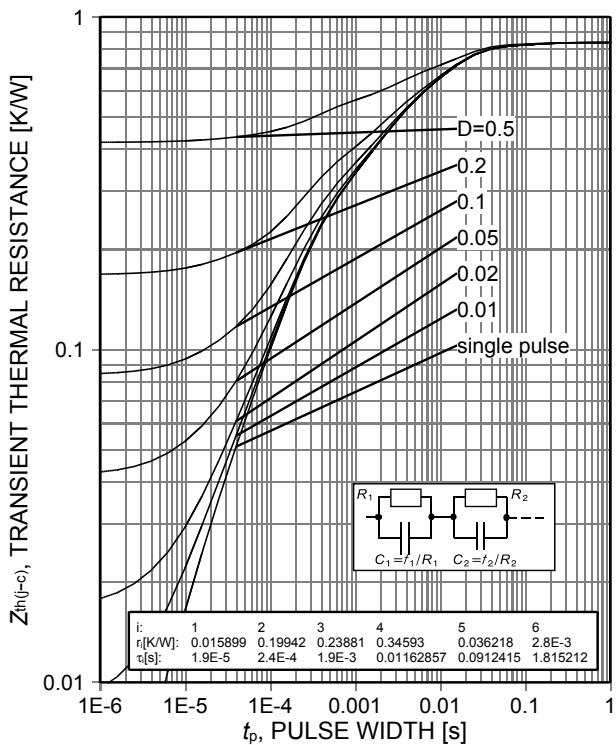
Figure 3. Diode transient thermal impedance as a function of pulse width
