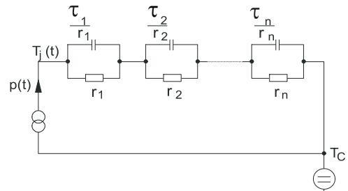
Figure D. Thermal equivalent circuit
