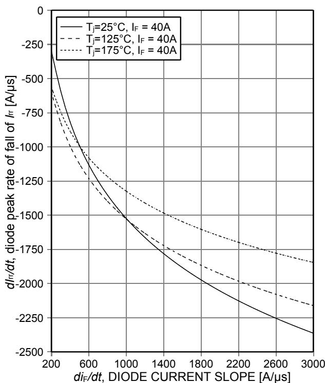
Figure 7. Typical diode peak rate of fall of reverse recovery current as a function of diode current slope
