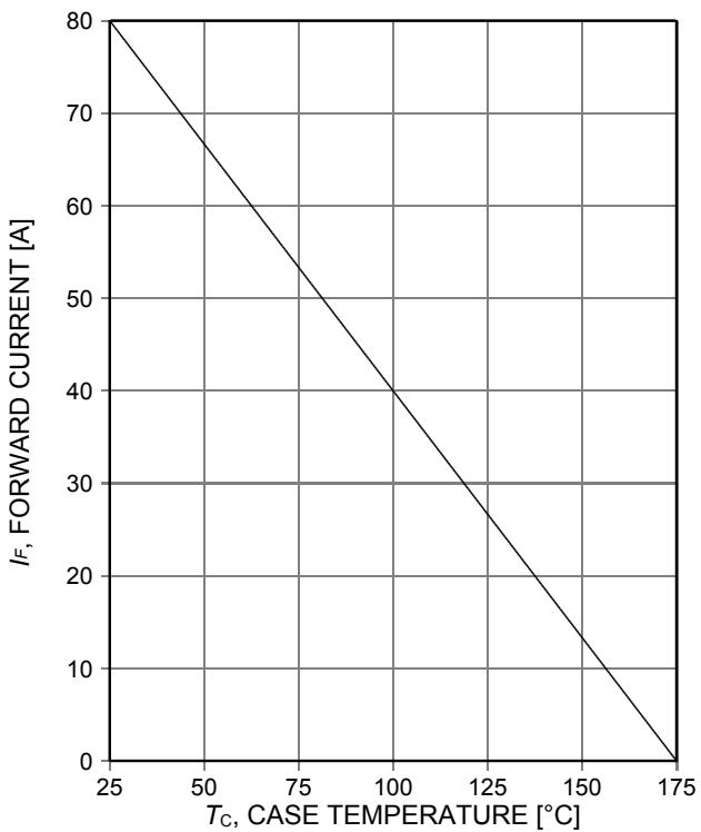
Figure 2. Diode forward current as a function of case temperature
