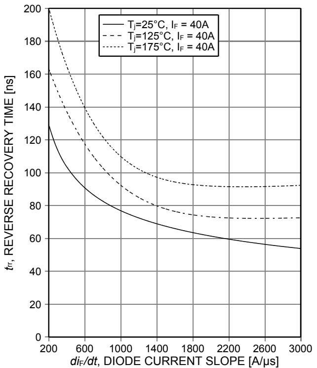
Figure 4. Typical reverse recovery time as a function of diode current slope
