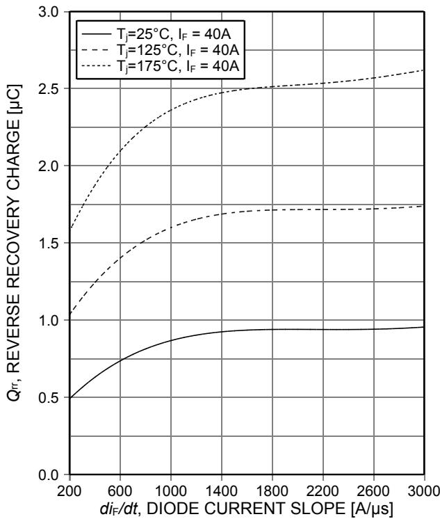
Figure 5. Typical reverse recovery charge as a function of diode current slope
