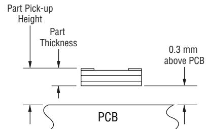
Recommended pick-up height: The bottom of the device should be 0.3 mm above the PCB.
