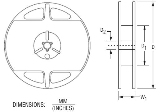
Devices are packed in accordance with EIA 481 standard specifications shown here.
