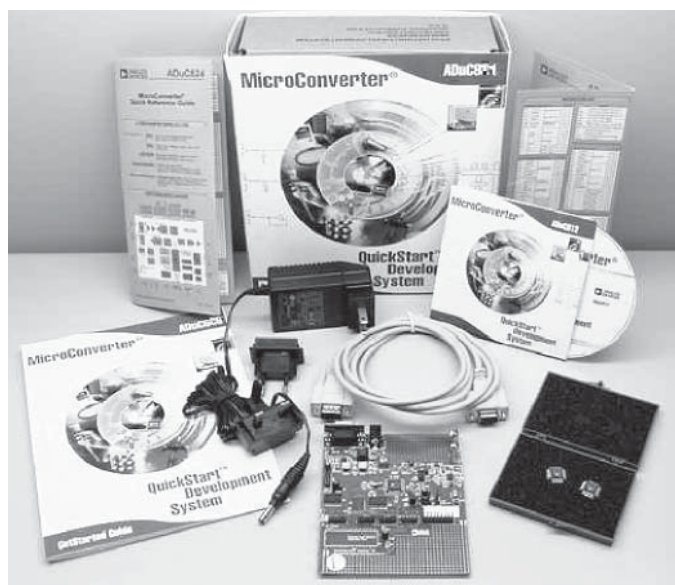
Figure 53. Components of the QuickStart Development System
