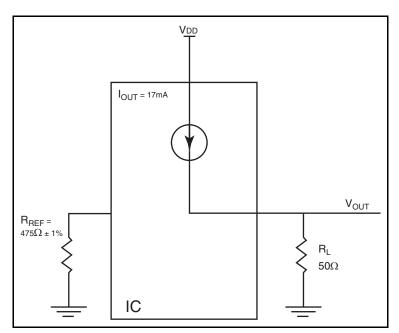
Figure 7. HCSL Driver Circuit and Termination
