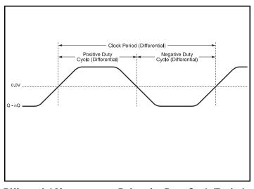
**Differential Measurement Points for Duty Cycle/Period**
