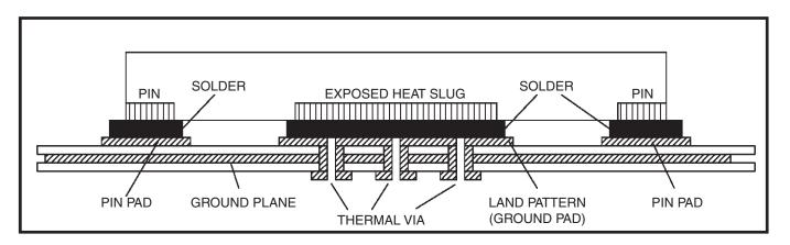
Figure 5. P.C. Assembly for Exposed Pad Thermal Release Path – Side View (drawing not to scale)
