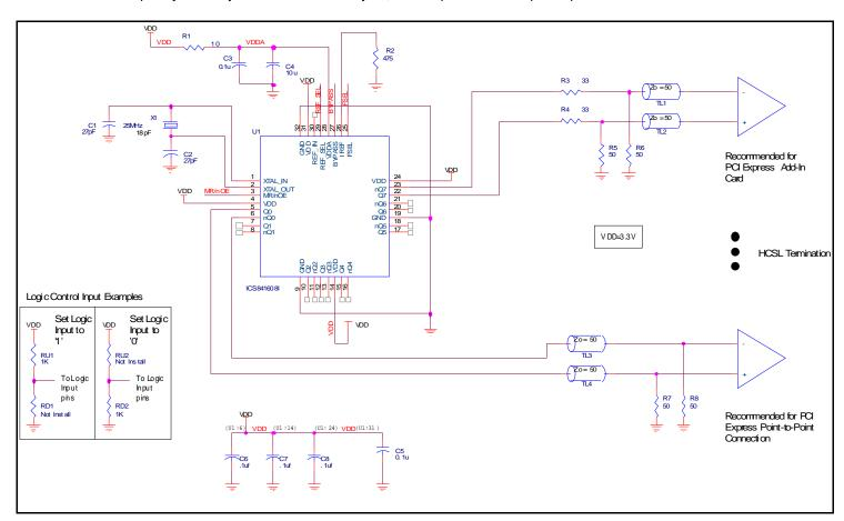
Figure 6. 841608 Application Schematic
