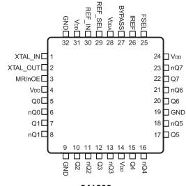
841608 32-Lead VFQFN 5mm x 5mm x 0.925mm package body K Package Top View
