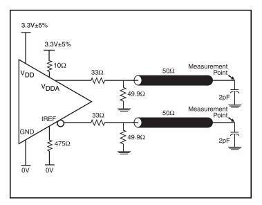
3.3V HCSL Output Load AC Test Circuit
