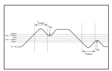
**Differential Measurement Points for Ringback**
