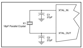
Figure 2. Crystal Input Interface
