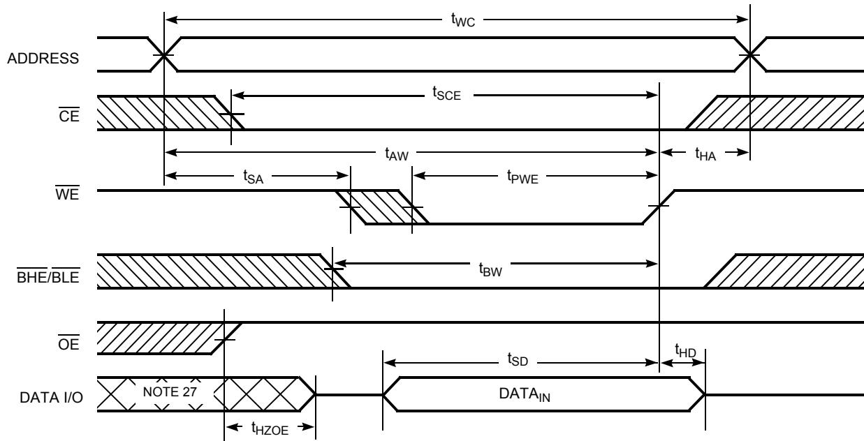
**Figure 7. Write Cycle 2:  $\overline{\text{CE}}$  Controlled** [24, 25, 26]
