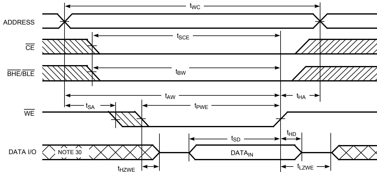
Figure 9. Write Cycle 4:  $\overline{\text{BHE}}/\overline{\text{BLE}}$  Controlled,  $\overline{\text{OE}}$  LOW [28]
