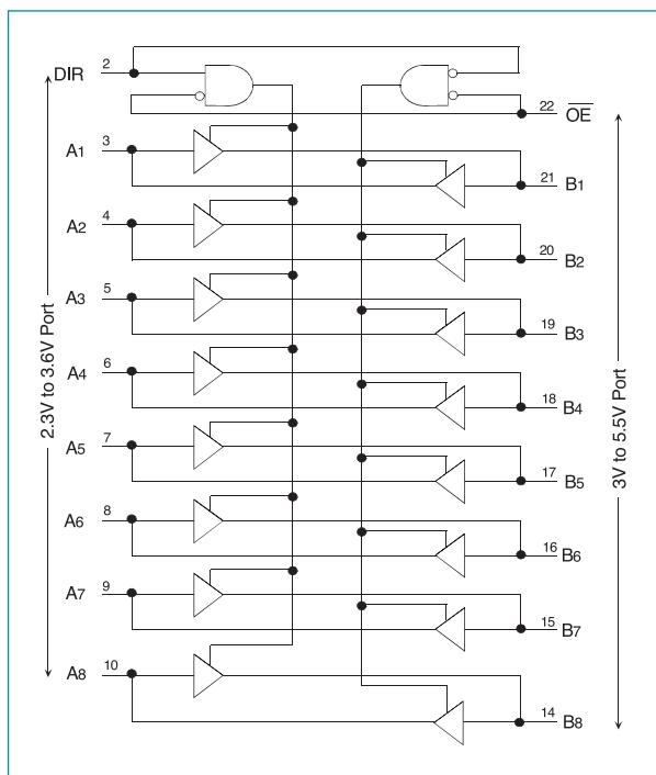
Figure 5: Block diagram of the 74LVCC3245 circuit
