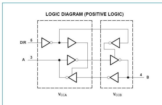
Figure 4: Block diagram of the 74LVC1T45 circuit
