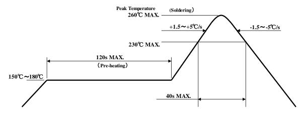
Notes 1 Temperature Profile for the reflow should be set to the surface temperature of resin which is on the top of LED. This should be the maximum temperature for soldering. Lowering the heating temperature and decreasing heating time is very effective in achieving higher reliability.
