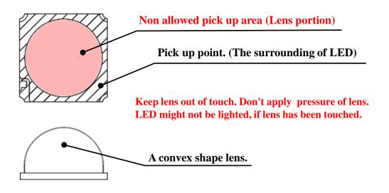
Please adjust the load, the pick up point, the nozzle diameter, etc. before mounting because the over load can cause the breakage of the surrounding of LED.
