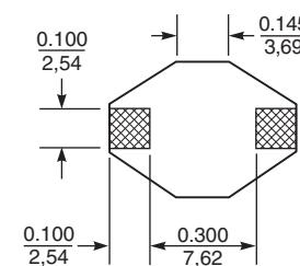
\*Allow an additional 0.02/0,508 in width and 0.01/0,254 in height for optional tin-lead and tin-silver-copper application.
