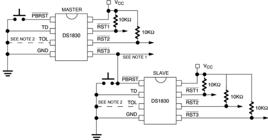
**Note 1:** The  $\overline{\text{RST3}}$  output tied to the pushbutton reset would be pulled to  $V_{CC}$  through the  $40\text{k}\Omega$  resistor in the pushbutton input. If a stronger pull-up is required an additional pull-up resistor could be added.
