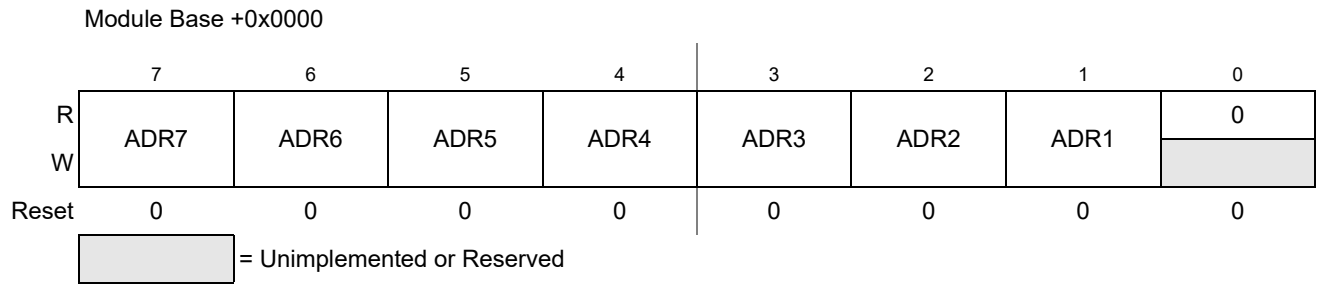
Figure 20-3. IIC Bus Address Register (IBAD)
