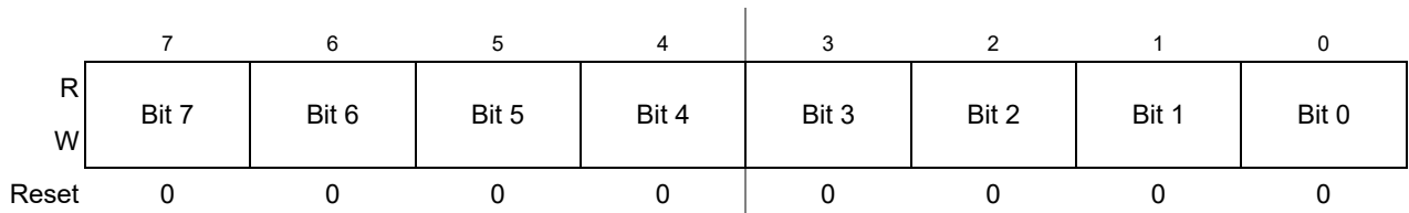
Figure 16-19. Timer Input Capture/Output Compare Register x Low (TCxL)
