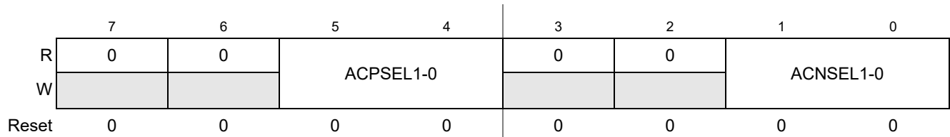
Figure 3-3. ACMP Control Register (ACMPC1)
