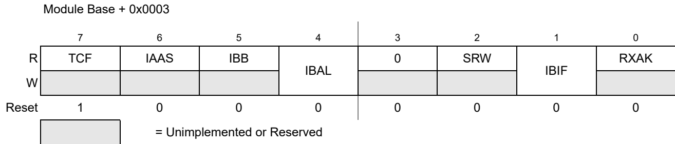
Figure 20-7. IIC Bus Status Register (IBSR)
