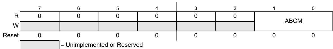
Figure 7-4. Debug Control Register2 (DBGC2)
