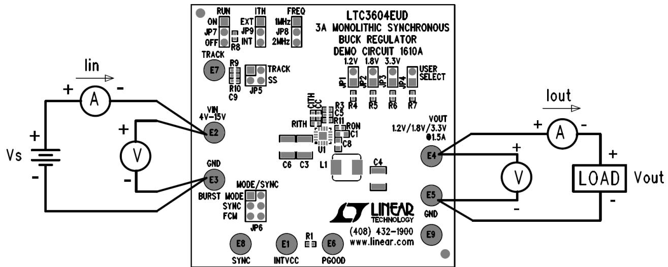
Figure 1. Proper Equipment Measurement Set-Up
