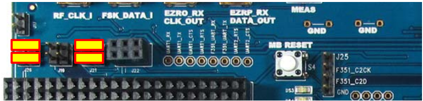
Figure 17. Radio Power Headers Diagram (EBID Powered by 5 V)
