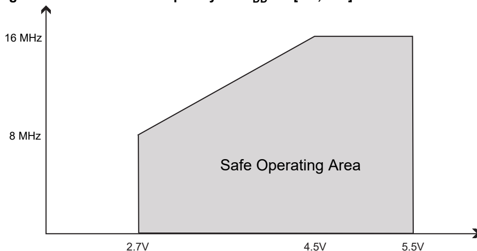
Figure 38-1. Maximum Frequency vs. V_{DD} for [-40, 125]^{\circ}\text{C}
